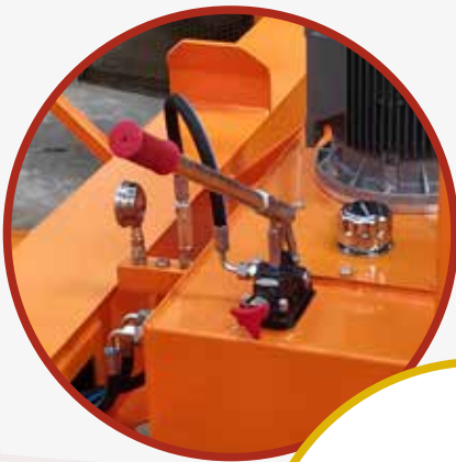
Emergency Hand Pump
